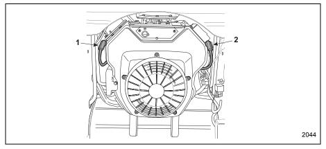
Figure 4-17 Check Spark Plugs and Cables
